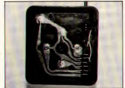
The circuit board in position in the base of the Atari joystick.
